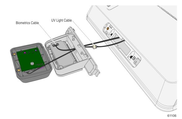
b. Rotate the UV Light module until it is detached.
