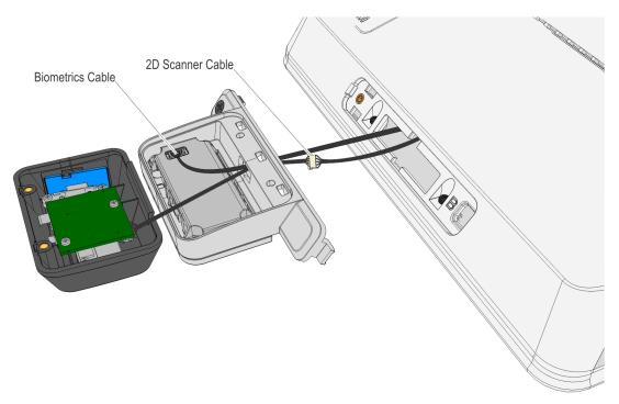
4. Snap the 2D scanner into the bracket. Ensure the snaps are fully engaged.
