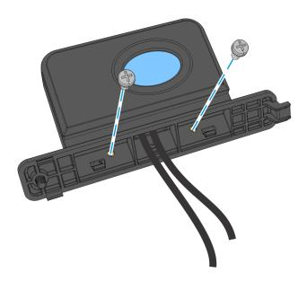
6. Gently push the biometrics and 2D scanner cables into the rear housing.
