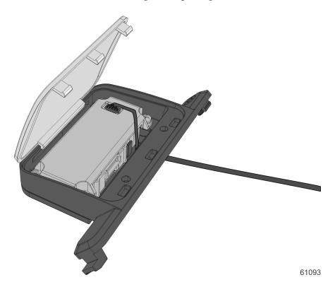
4. Snap the bottom blank into the bracket. Ensure the snaps are fully engaged.
