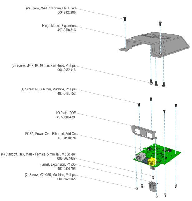
This kit provides the components to add a POE + SIM + RJ45 Expansion.
