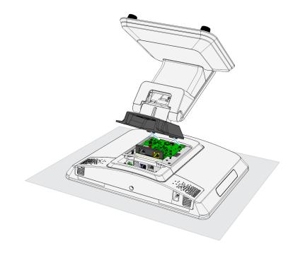
6. Secure to rear housing with screws (2).
