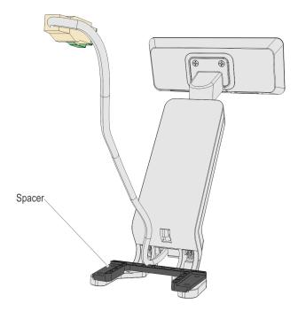
Route the cable from the customer display up through the P-Series stand and install the Spacer and customer display onto the bottom of the stand. Secure with screws (4).
