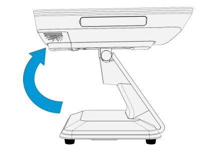
2. Remove the Upper Stand Cover by pivoting it away from the stand. The cover has a simple snap fit connection at the top.
