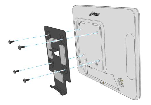
5. Install the Bracket onto the back of the customer display.
