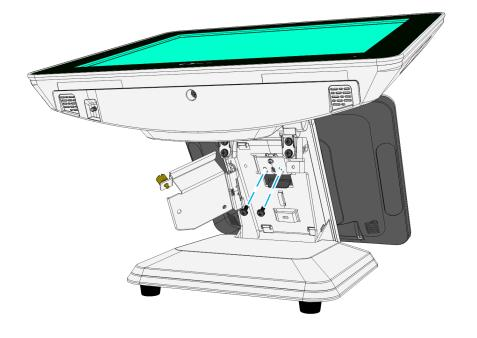
b. Pivot the assembly into position on the P-Series Stand and secure it from the inside with screws (2).
