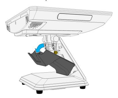
3. Loosen the thumbscrew to open the Cable Door.
