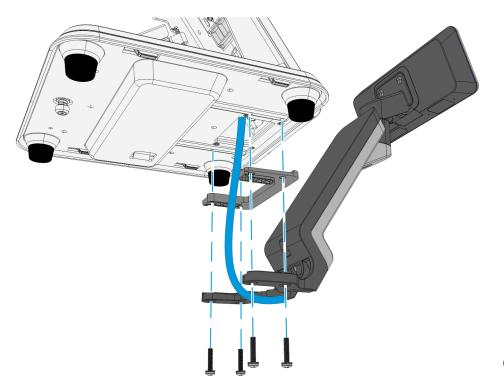
5. Loosen the screw on the Terminal Cable Cover. To open, press on the indentations in the Cable Cover to unlatch the cover and then pivot the cover open.
