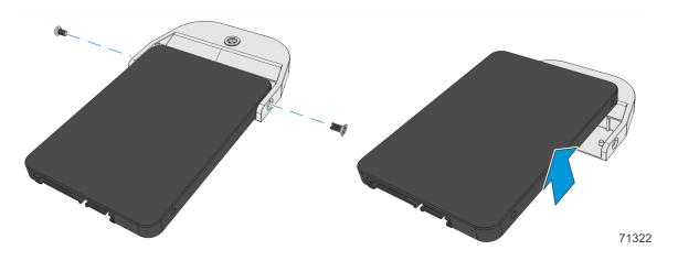
6. Mount the new 40GB/60GB/120 SSD to the Solid–State Cover through the keying features. Secure with screws (2).
