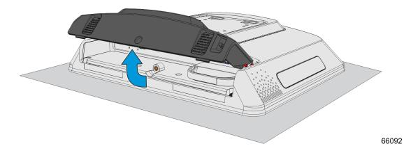
3. Remove the screw (1) that secures the Solid–State Cover.
