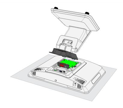
6. Secure to rear housing with screws (2).
