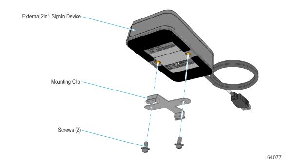
3. Snap the mounting clip to the plate to secure assembly.
