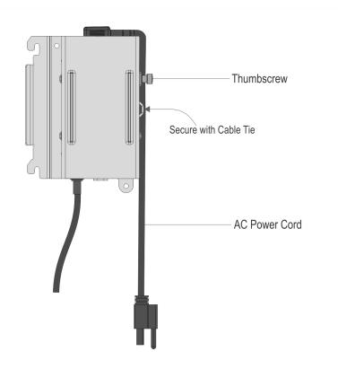
4. Secure the bracket with the thumbscrew and the AC Power Cord with a cable tie.
