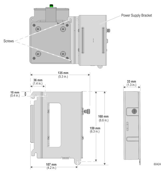
2. Insert the power supply into the bracket (AC Connector on top).
