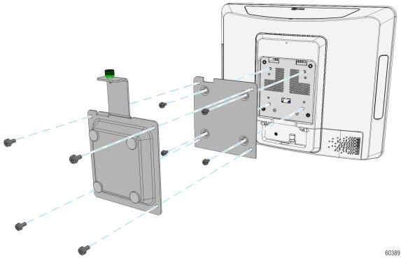
2. Secure the Mount Plate (with UP arrow pointing up) to the vertical surface using lag screws (4). Make sure you install the screws into the studs or that you use hardware of similar strength. Use the bracket as a template to mark the location of the holes or use the dimensions shown below.
