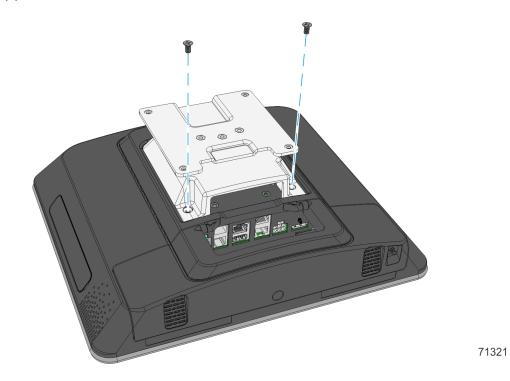
4. Attach SpacePole mount with standard flat mounting plate to P–Series POS display with Expansion assembly. Secure with M4 x 8 screws (4).
