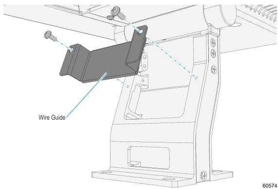
4. Route the cable behind the wire guide down to the pole mount base.
