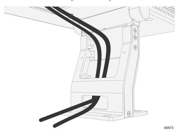
5. Replace the wire guide and secure with screws (2).
