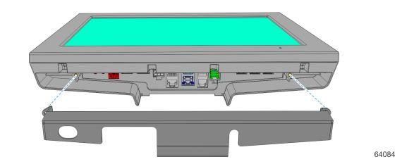
3. Secure the tamper proof cover with screws (2).
