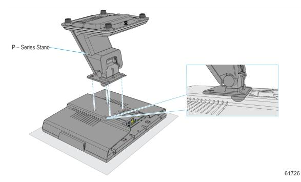
2. Secure the Hinge Mount with screws (2) on the bottom holes.
