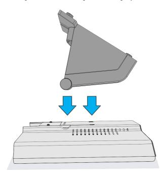
2. Secure the Table Top Tilt Stand with M4 x 30 screws (4).
