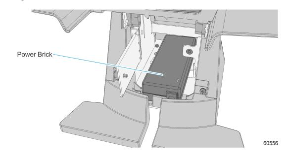
5. Route the AC power cord to the right of the power brick and then down the opening at the base of the terminal.
