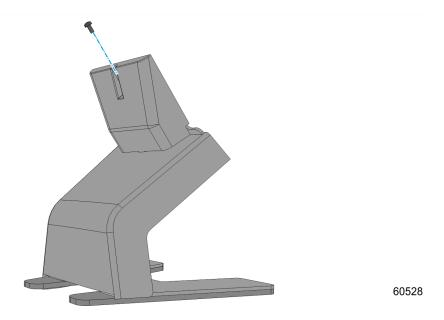
2. Remove the Back Connector Cover.
