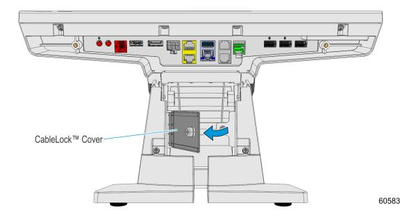
9. Route the cables under the stand and up through the CableLock<sup>TM</sup> Cover.
