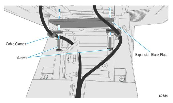
**Note:** If the POS includes an expansion, install the cable clamps under the expansion and secure with screws (2).
