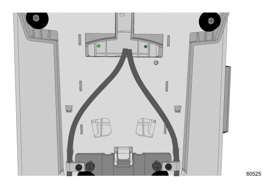
11. Route the cables under the stand and up through the CableLock<sup>™</sup> Cover.
