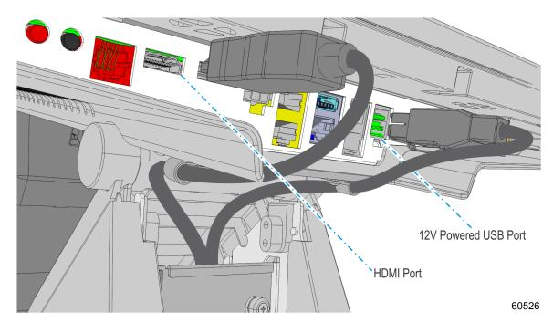
15. Connect the cables to the HDMI and 12 V Powered USB ports.
