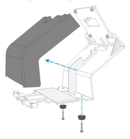
3. Remove the screws (2) and rubber foot (2). Remove the Stand Cover.
