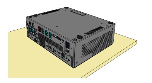
2. Install the Bracket and Rubber Feet Assembly on the CX8 (2 screws per assembly).
