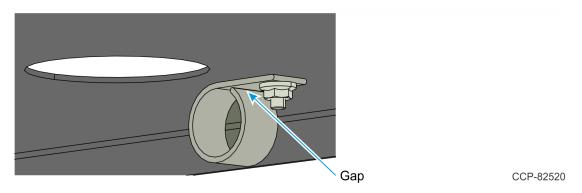
4. Route the scale cable through the Top Tray opening and through the P-loop as shown.
