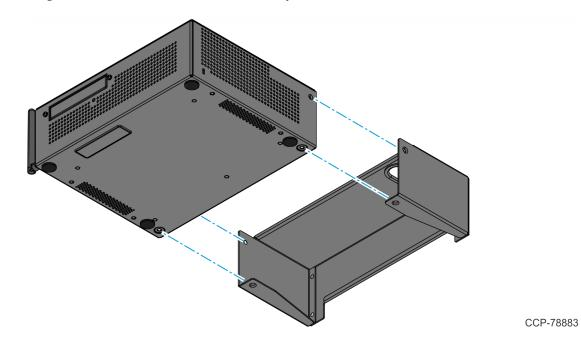
2. Align the screw holes of the I/O Security Cover with the screw holes of the chassis.
